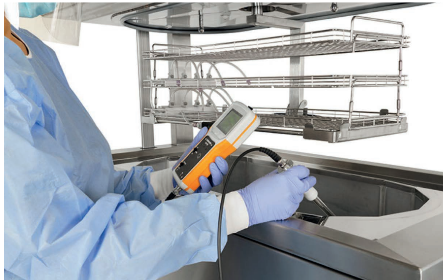
Fig 2 Technician measuring cavitation with CVD
