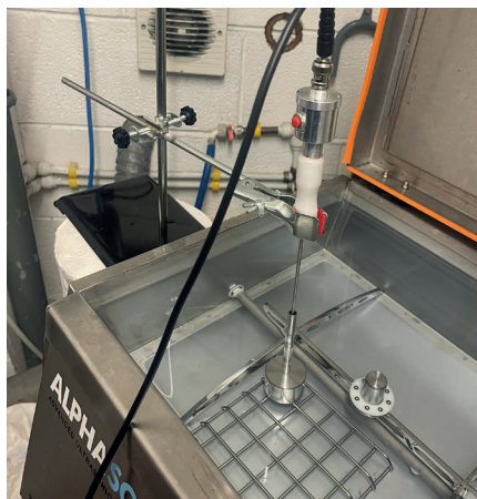
Fig 3 Cavitation Validation Device measuring ultrasonic losses in a simulated lumen
